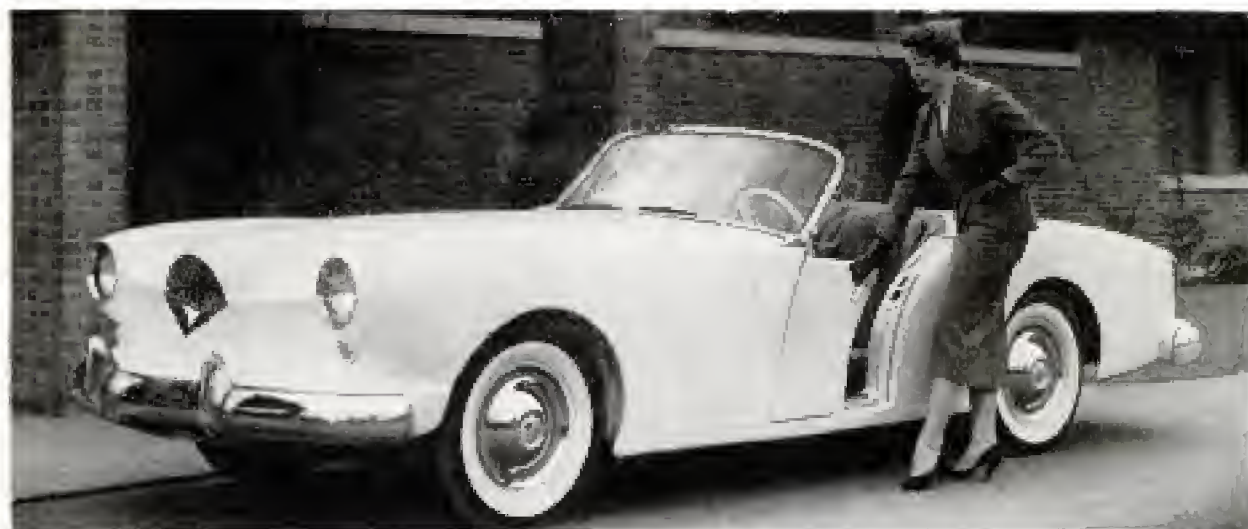
Doors on the sleek Darrin slide forward into the body. The base of the windshield is only 36 inches high
